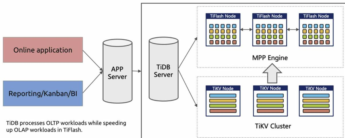
TiDB initially processes a write request to the row store. From there, it is replicated to the column store. Data is written first to TiKV, which is the row store. TiKV provides the speed needed for massive OLTP. Next, the data is replicated to TiFlash, the column store. Data replication is peer to peer with no in-between layer, so the data is replicated in real-time.
