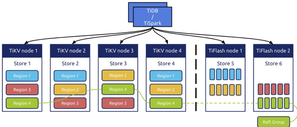
TiFlash uses a Massively Parallel Processing (MPP) engine. MPP is a storage structure designed to handle multiple operations simultaneously by several processing units. Each processing unit works independently with its own operating system and dedicated memory, meaning each node in a cluster works independently, consumes resources (CPU, Memory, Storage) from its own nodes, processes data on its own nodes, and does not share any data or resources with other nodes.
